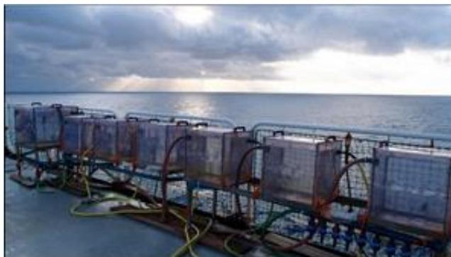
**Figure 1.** Photograph of the incubators on board the R/V Marion Dufresne, equipped with light filters and supplied by surface seawater to maintain representative radiance and temperature of the surface ocean
